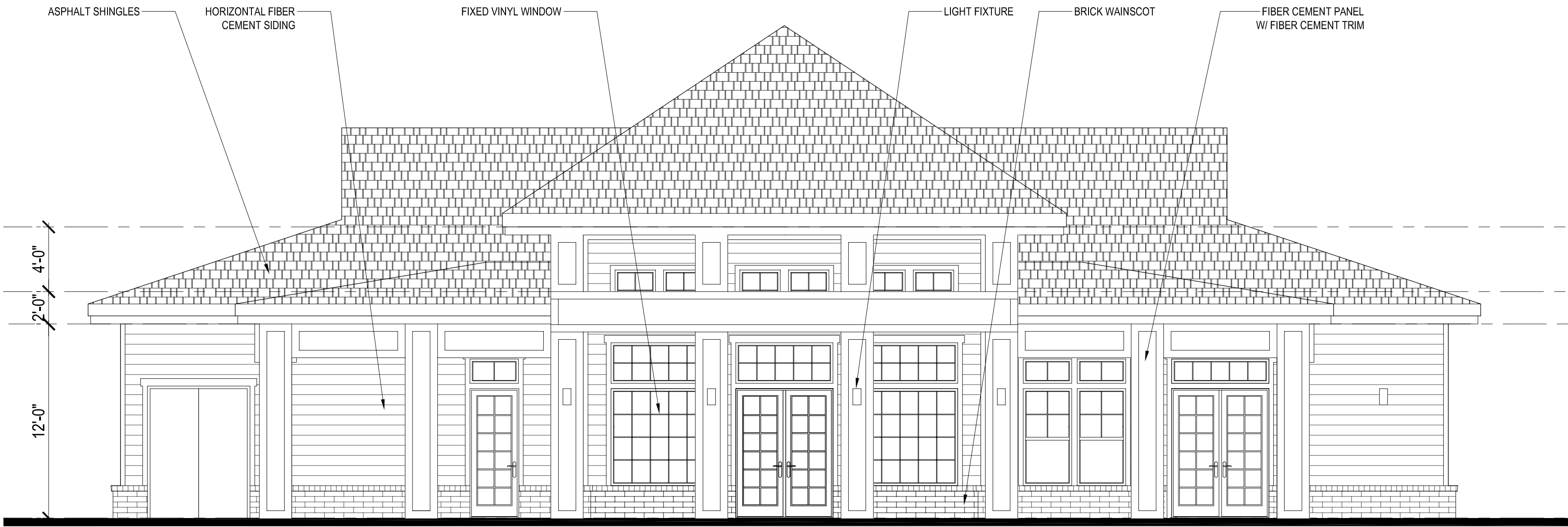
2 CLUBHOUSE - SOUTH ELEVATION SCALE: 3/16" = 1'-0"
